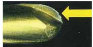
No.3 (C) 超硬エンドミル (2個加工後) No.3 (C) TC Endmill (after 2pcs. Cutting)
