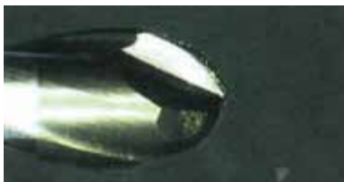
No.1 (A) c BNスパイラル刃エンドミル (6個加工後) No.1 (A) c BN Spiral Endmill (after 6pcs. Cutting)
