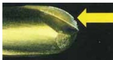
No.3 (C) 超硬エンドミル (2個加工後) No.3 (C) TC Endmill (after 2pcs. Cutting)
